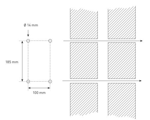
Make a recess of  $140 \times 230 \times 140 \text{ mm}$  (bxhxd) in the outer wall to hold the façade plate/roll (140 mm deep). The lower incision must face downwards at an angle. Turn the thread ends into the sleeve of the façade plate. Push them through the wall. Draw on the thread ends so that once you have sawn them off they still stick out by 3 centimeters.
